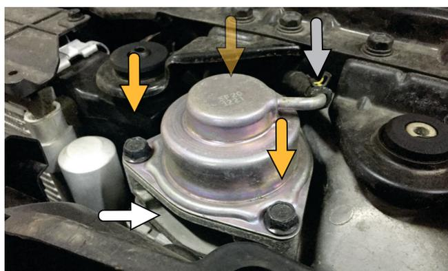
The factory vacuum hose needs to be replaced with the supplied hose to reach the DVX vacuum port.
